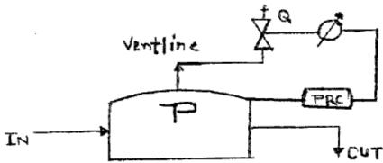
Is controlled by a digital (discrete time) proportional controller of gain Kc. The measurement from the pressure sensor is sampled every 60 secs, for the transmission Via a ZoH element to controller which is connected directly to a control valve on a line which vents the vessel. The transfer function representing the process i. c. between P and the flow rate Q through the vent
