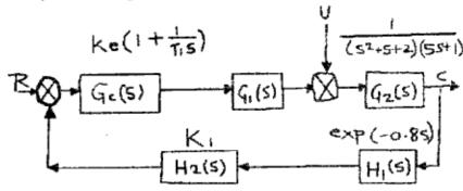
The transfer function describing the various blocks with Kc = 10,  $T_1 = 60$  sec  $K_1 = 0.8$  and K = 0.5. By determination of the gain and phase margins, show the effect on the stability of the control system of introducing the derivates along with  $T_0 = 60$  sec.
